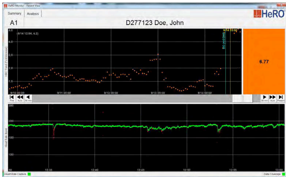
Figure 1. HeRO Patient View. The Patient View displays a five-day trend of the HeRO Score and a 30-minute trend of heart rate data. In this example, a positive blood culture is preceded by a rising HeRO trend, while the heart rate trend shows low variability punctuated by very subtle decelerations.
